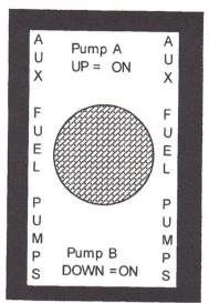
4. Procedures Placard 12/24-58 located on the instrument panel in full view of the pilot:
